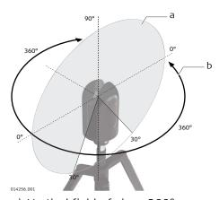
a) Vertical field of view: 300°b) Horizontal field of view: 360°
