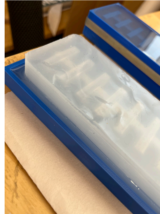
Dip Exposed Side of Part in Uncured Resin To Seal Armature
