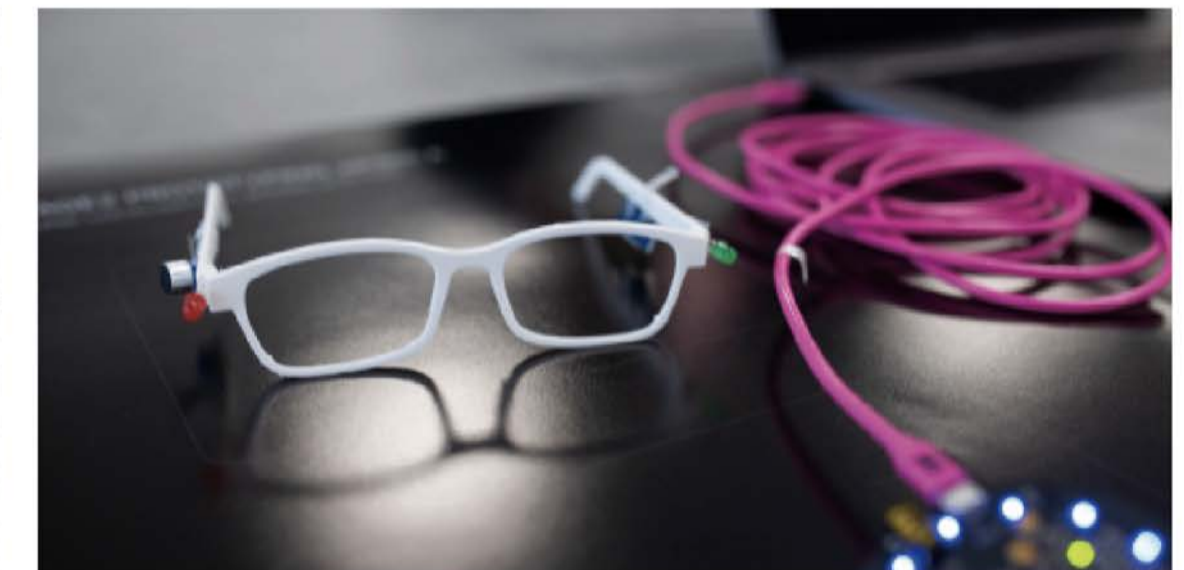
Fig. Prototype I, LED indication glasses
