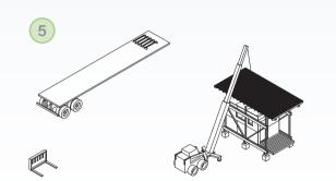
LIFT ROOF ONTO TRUSSES WITH SKIDSTEER CRANE ATTACHMENT
