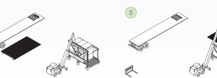
LIFT TRUSSES ONTO COLUMNS WITH SKIDSTEER CRANE ATTACHMENT
