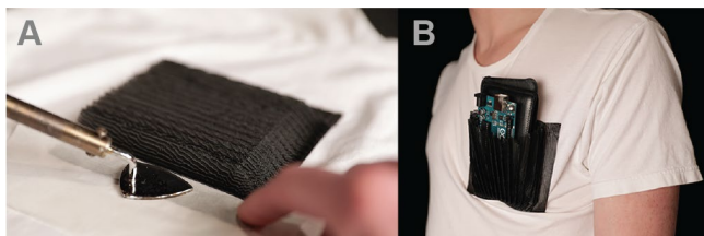
Figure 9: A) The pleated DefeXtile pocket is bonded to the shirt with an iron. B) The pocket supporting the weight of a phone, wallet, and Arduino board.
