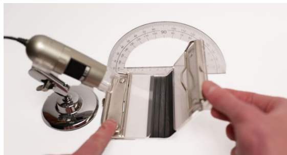
Figure 14: Bend Testing of PLA DefeXtiles. A microscope was used to help monitor crack initiation.
