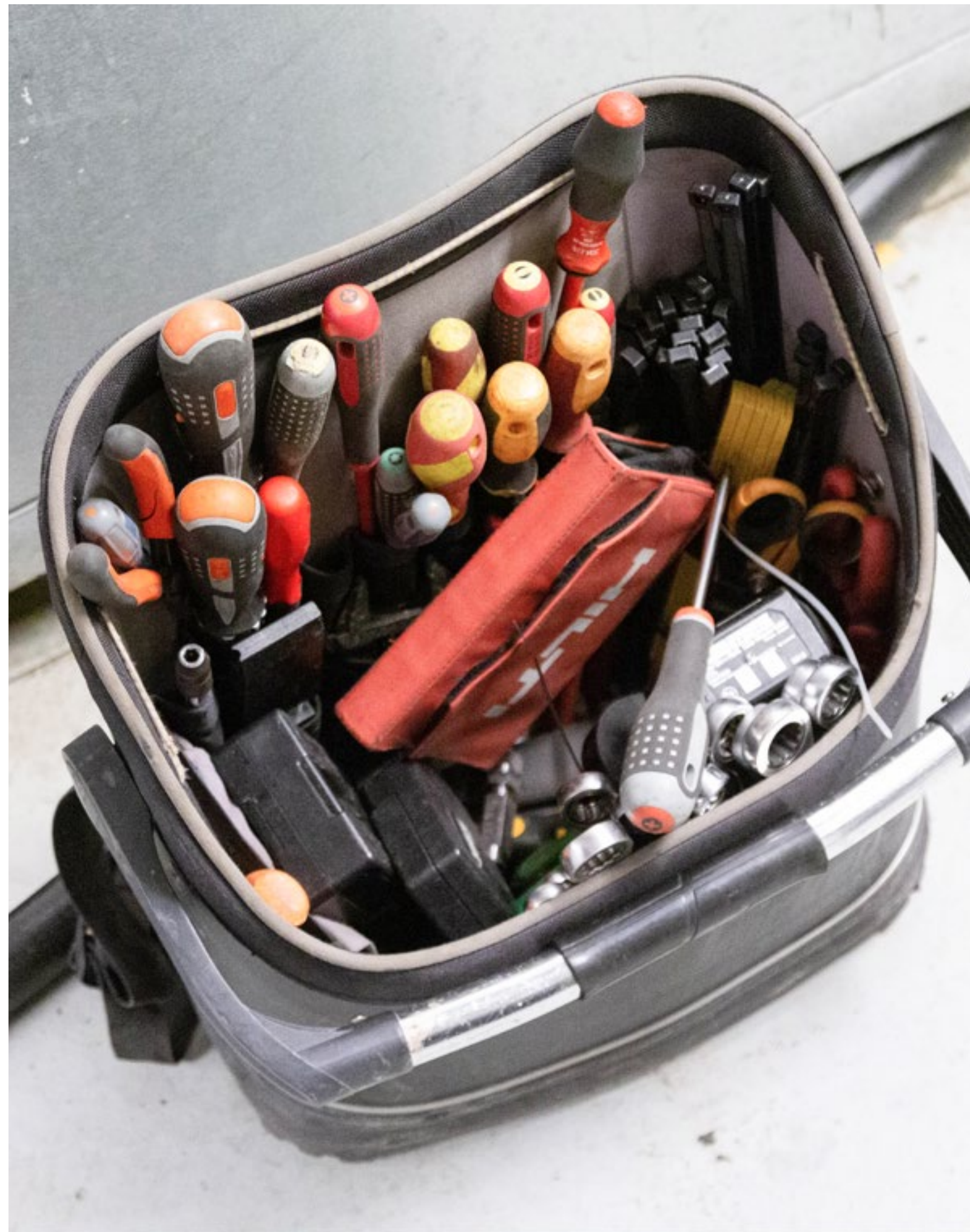
The main toolbox holds frequently used smaller tools like screwdrivers and wrenches within reach when working on the ground. These tools are some of the most commonly used when maintaining a mast. The necessary tools are transferred to a toolbag when working aloft.
