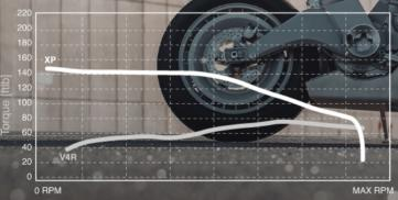
2020 Zero SR/F - max 146.45 ftlb / 198.56 Nm @ 1,218 rpm\* 2019 Ducati Panigale V4R - max 76.65 ftlb / 103.92 Nm @ 12,300 rpm\*
