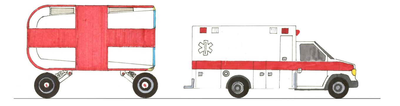
The unit would be a similar scale to traditional ambulances when closed, but provides a better suspension system that could allow for operation outside of city infrastructure
