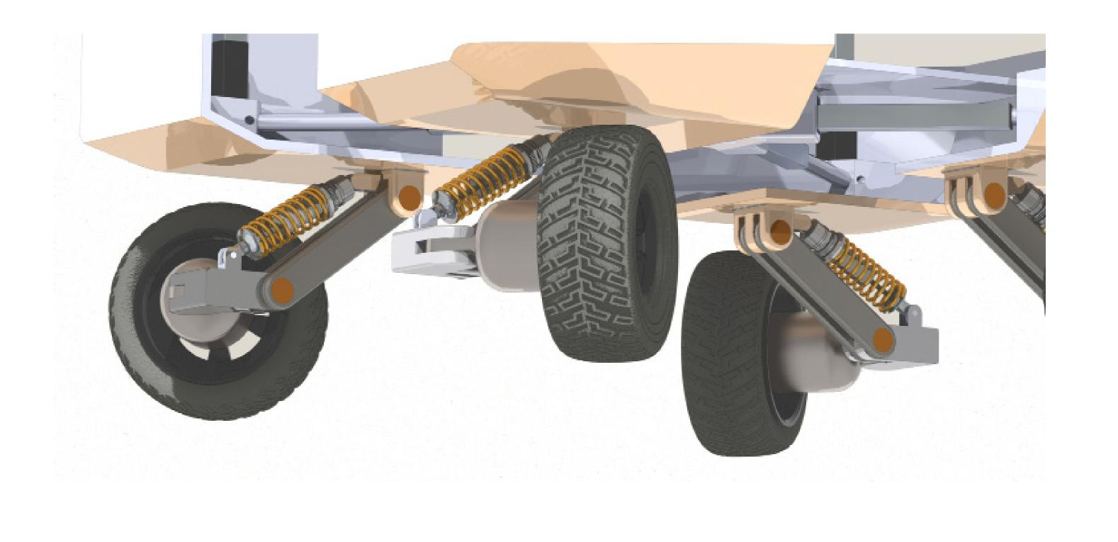
Motorized hinges allow the wheels to rotate 45 degrees in order to drive the expansion mechaanism outward. The hinges also solve the steering problem associated with independent drive sysytems.
