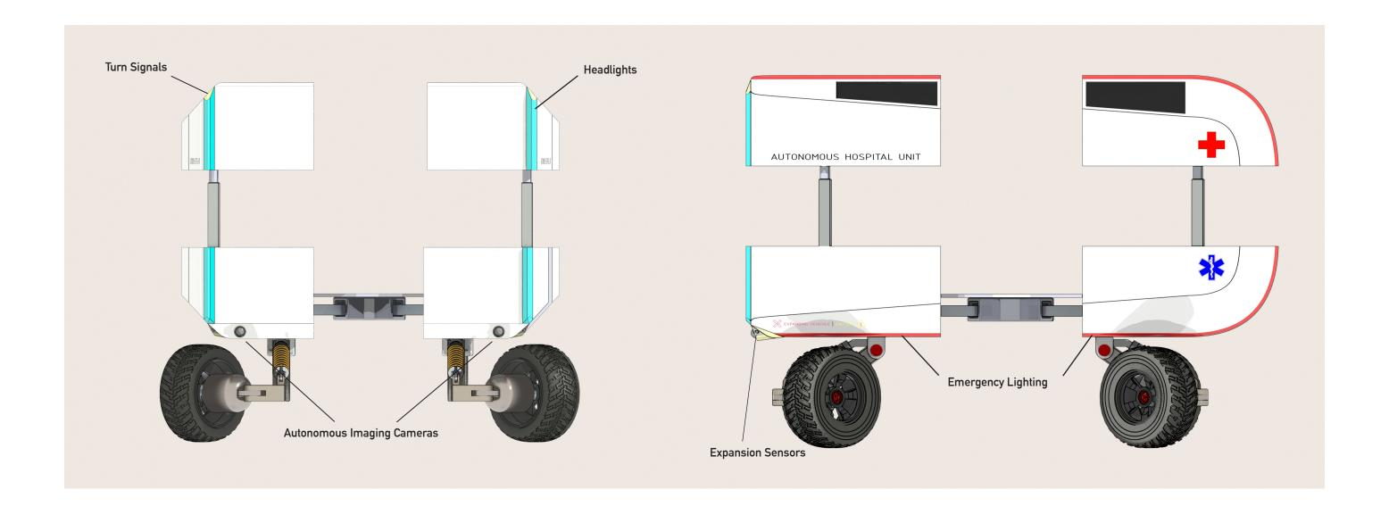
Once all wheels have rotated 45 degrees, the unit senses the surrounding environment. Using equiped imaging technology, it scans its perimiter for any obstructions.
