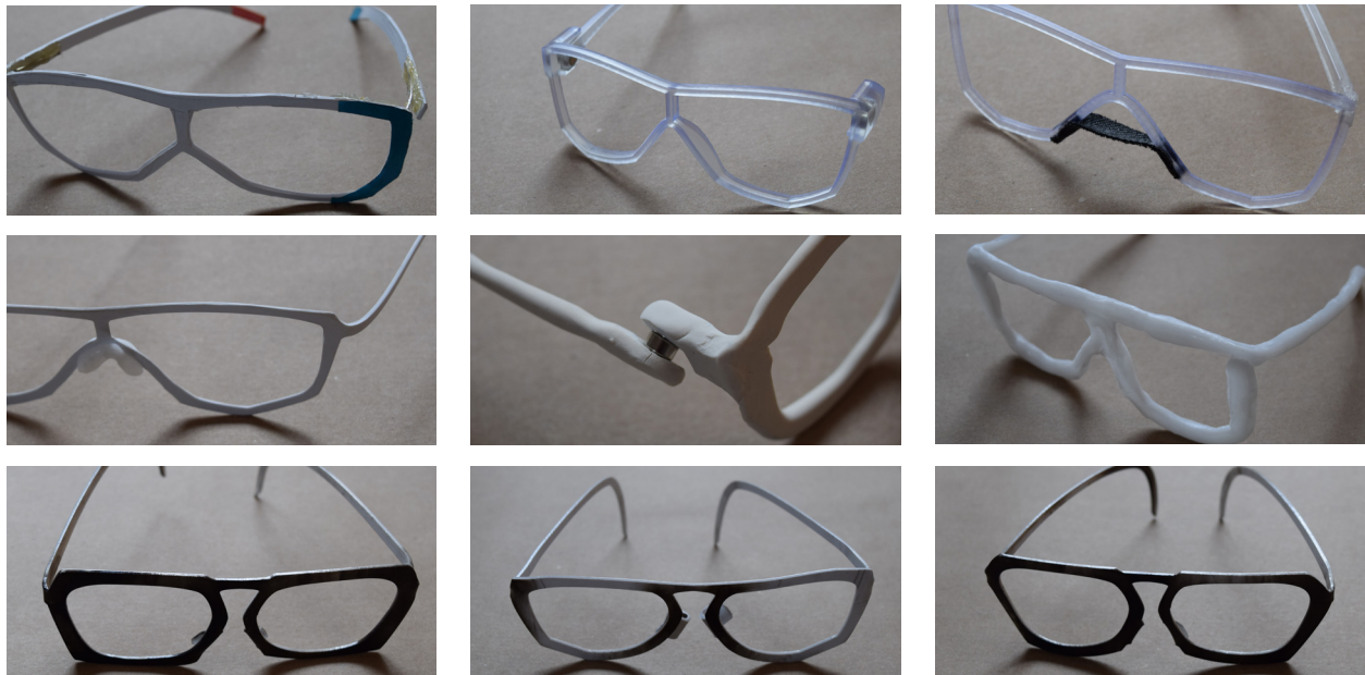
FIG. 7 Prototypes of fabric and thermoplastic nose pieces, and wire, magnetic, and thermoplastic hinging mechanisms. Photos by the author.
