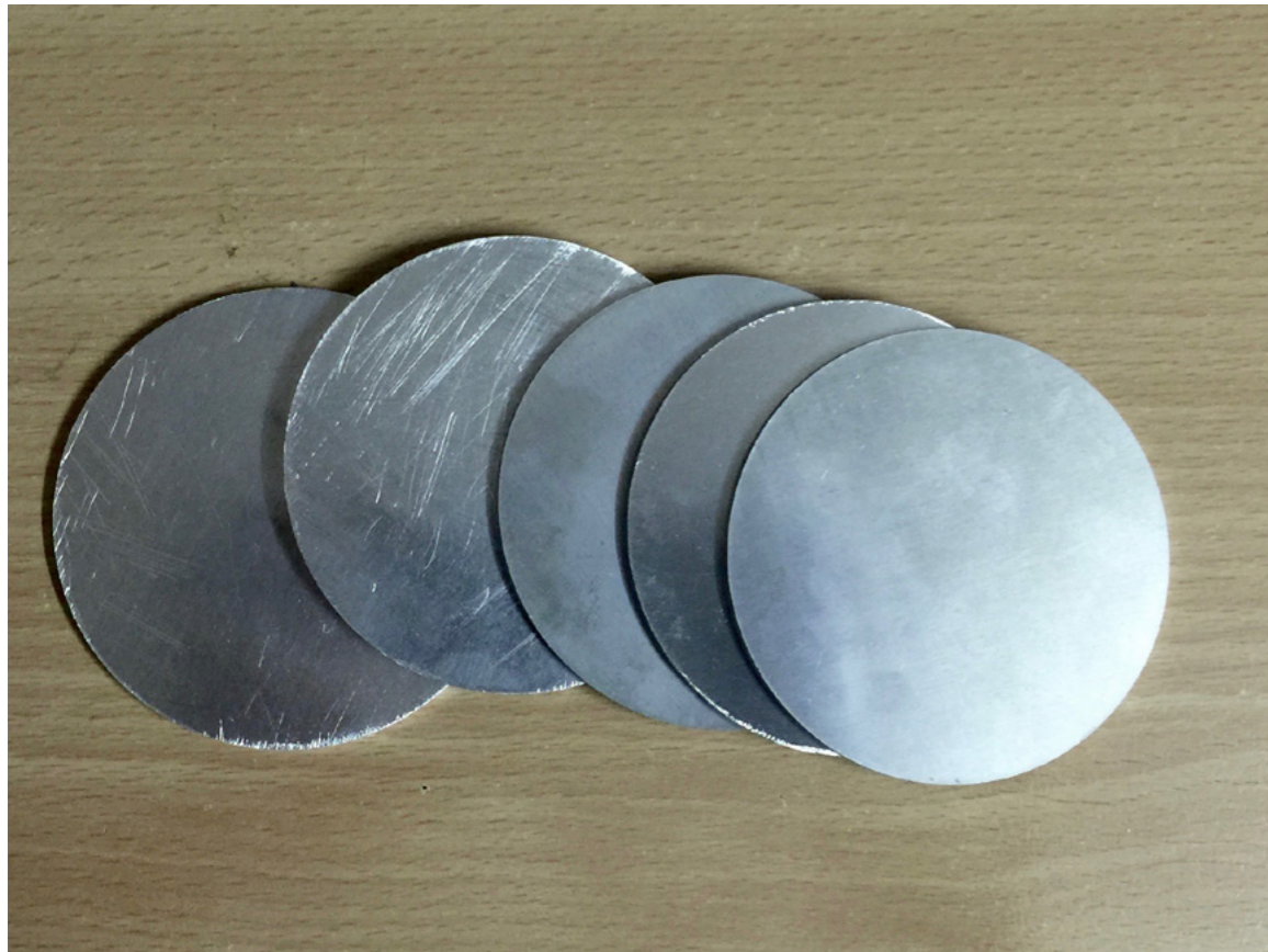
Images from L to R Aluminium circles cut via laser cutter Collin's Anodic treatment samples Anodised Aluminium circles
