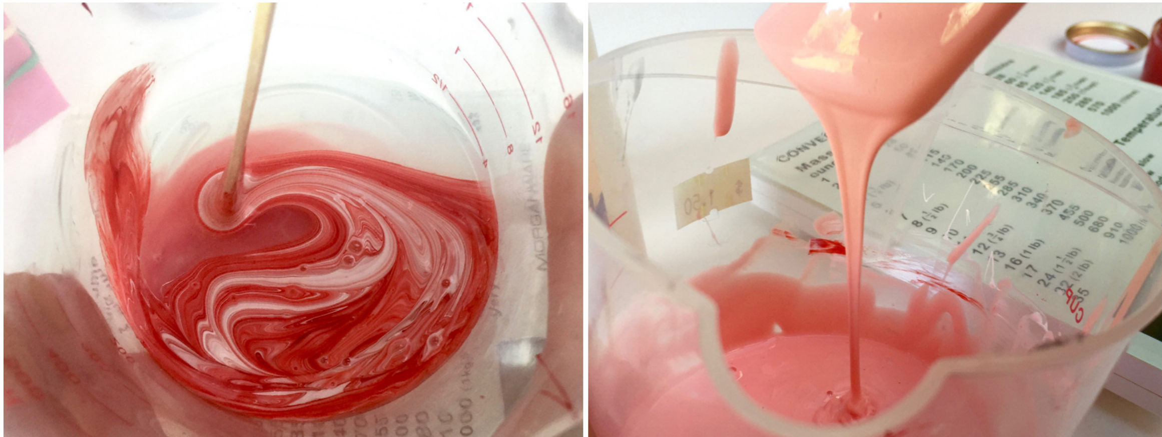
Process of adding pigment into silicone and injecting it into the pinksil mould
