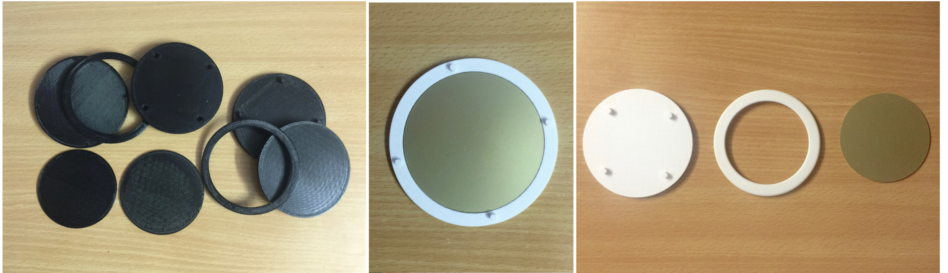
Images from L to R 3D print trial and errors Fitting the anodised aluminium circles into the best fitting face plate
