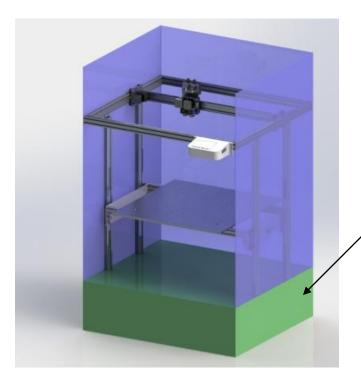
Increase the height and use space for filament and power supply, etc
