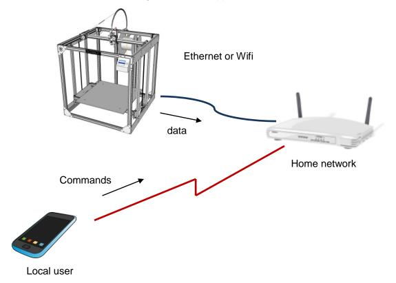
It is also possible to run the single board computers network in ad-hoc mode. This requires no external network or router. You wifi device can connect directly to the Gigabot.
