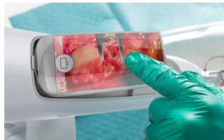
Using cameras and LED light, a clear view of the operation field is transported from the tip of your instrument to a high resolution screen in your field of vision.
