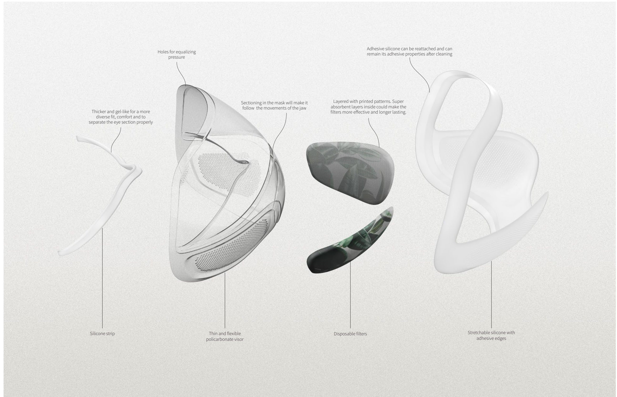
The reusable and full facepiece respirator with disposable filters prevents the three ways of transmission: inhalation of aerosols, droplet and contact. It consists of a light plastic visor which is combined with adhesive and stretchy silicone. The soft and gentle adhesive edges makes it more effective and safe than disposable respirators by completely sealing the edges to the face.
