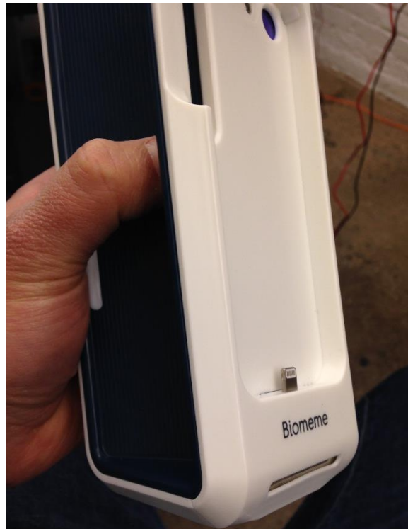
The one3 without an iPhone docked. The hinged Lightning connector allows wireless data transfer and direct charging of the iPhone, without having to remove it between tests.
