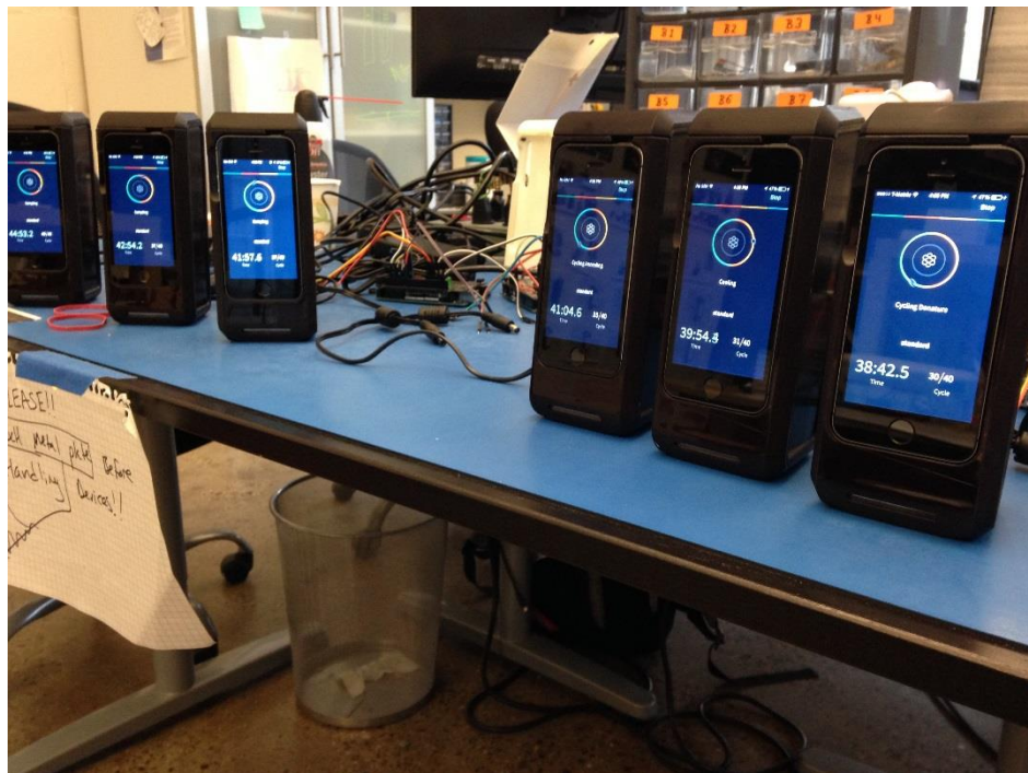
Rapidly produced stereo lithography housings enabled beta testing while plastic injection molding tools were fabricated.
