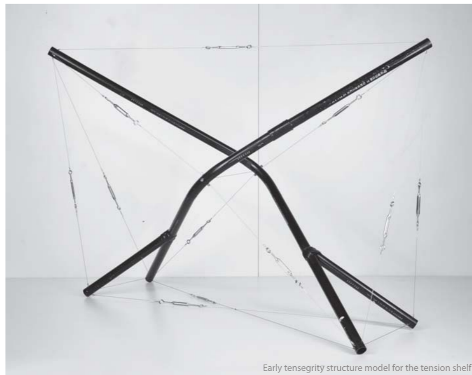
Early tensegrity structure model for the tension shelf
