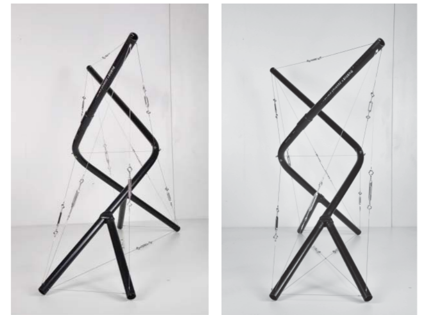
Early Tensegrity Structure | PVC Pipe & Stainless Wire L1200*D400*H900_mm
